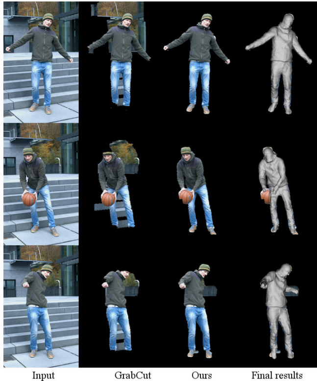
Fig. 12. Robustness of our model based silhouette extraction method. Our model based silhouette extraction method yields significantly more accurate foreground segmentation results than the default GrabCut method. Our correspondence prune strategy improves the robustness of our silhouette based surface refinement to segmentation errors (row 2). The failure case, in which the pose estimate is far off, cannot be corrected by our silhouette based refinement (row 3).
